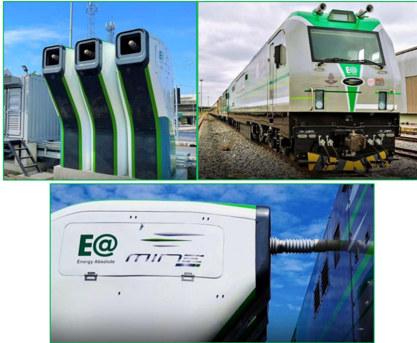
EA's 1 MW Megawatt Charger supporting electric locomotive operations under the MINE E- Locomotive project.
